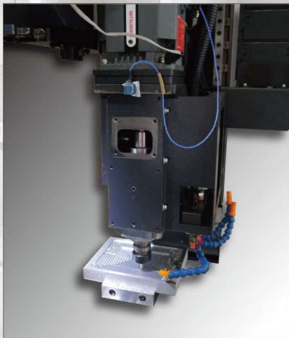
Spindle Vibration Test in Y Direction
